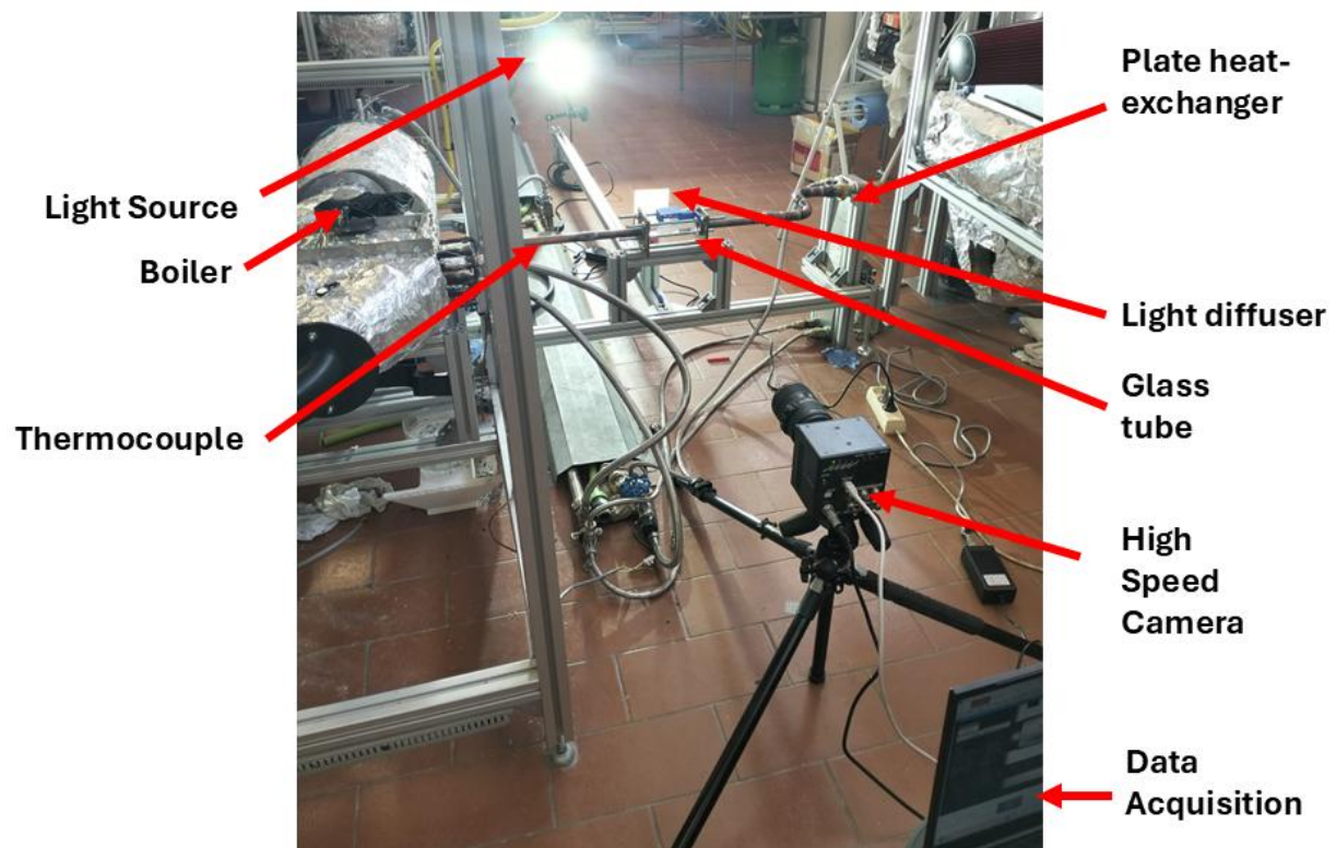
Figure. 1 Two-phase boiling-of-water flow visualization experiment.
