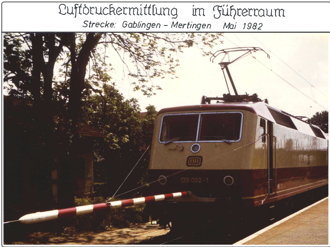
Figure 3. Boom-mounted wind probe used on the German national railway (1982). Title translation: "Measurement of the dynamic pressure from the driver's cabin". [ Image graciously provided by Dr. Thorsten Tielkes (DB Systemtechnik, Germany) ]
