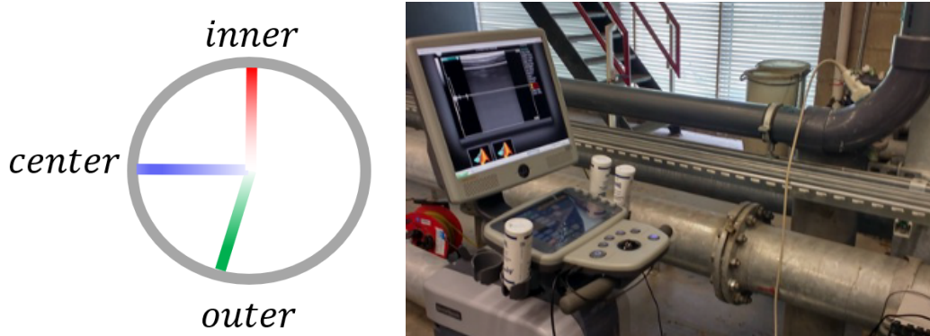
Figure 3: left: orientations of measured velocity profiles, right: detail of experimental setup.
