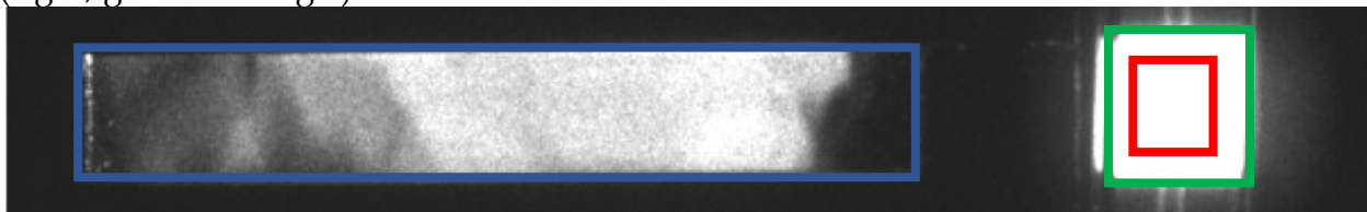
Figure. 3 Raw LIF image in the second void (Pos. 3) of layer L14 for Re_p = 99 and Q_{jet} = 2 \frac{1}{\text{min}} . The anisole distribution in the optical module is shown on the left hand side (blue rectangle) and the anisole in the flow cell on the right hand side (green rectangle).
