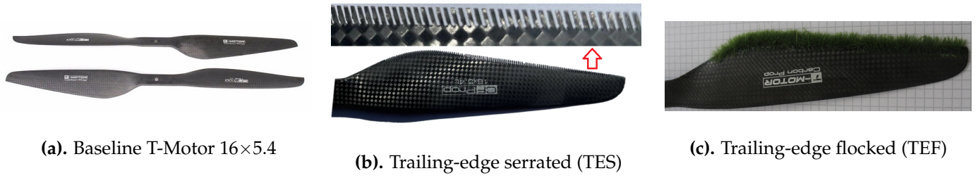
Figure 2. Baseline propeller and trailing-edge modified variants.
