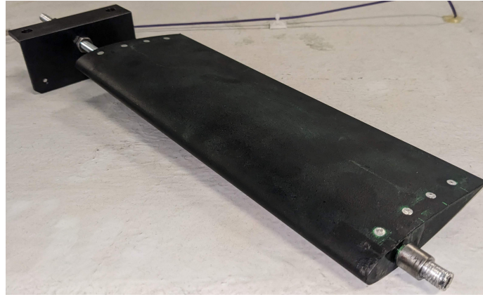
Figure 3. NACA 0018 airfoil model with fiducial markers and support.
