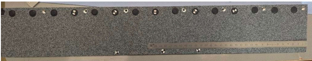
Figure 2. Stainless steel seal with printed IPCT pattern.
